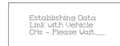
If the EOBD function is selected, the screen will prompt you to turn the ignition on and then press the ✓ key. The hand-held tester will automatically establish communication with the vehicle's On-Board Diagnostics.
