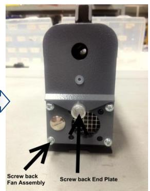
Screw back Fan Assembly Screw back End Plate
