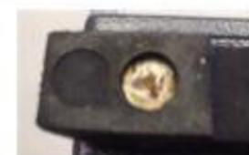
**Bad** The contact shown left is showing bad signs of arcing and corrosion and should be replaced.
