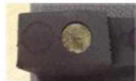
**Poor** The contact is slightly corroded through contact with dirt etc. Also, small signs of pitting of the plating.
