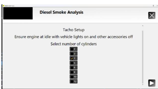
Check that the engine has reached operating temperature. Ensure all other accessories, internal blower, screen heater etc. are off but turn on the vehicle headlights. Allow the engine to idle while the CDSS6 initialises, approximately 17 seconds. When complete the unit will read engine speed on the bar graph.
