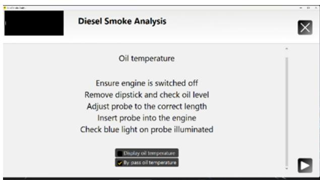
This will force a 40-second countdown before the procedure continues. However, it is imperative that the engine is fully warmed up before proceeding. Selecting further warm up will take the operator to an additional screen displaying engine speed to allow additional warm up of the engine if required.
