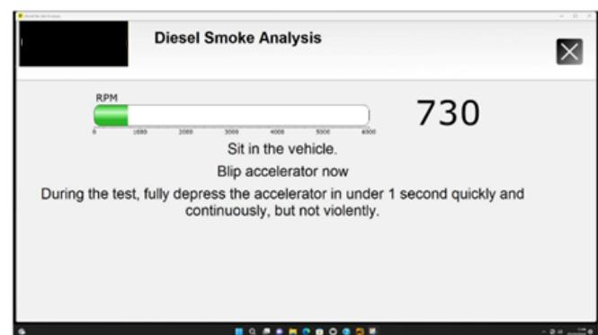
3. When instructed fully depress the accelerator pedal and hold.
