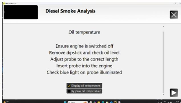
11. Select 'Display.....' or 'Bypass ' then click the PROCEED icon to continue. The screen will then display the measured oil temperature.
