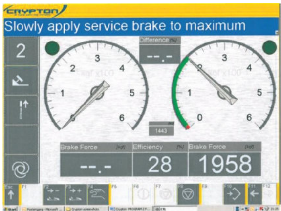
Save results with remote control F10 once maximum is achieved. Then press the associated button to start rollers to drive out.
