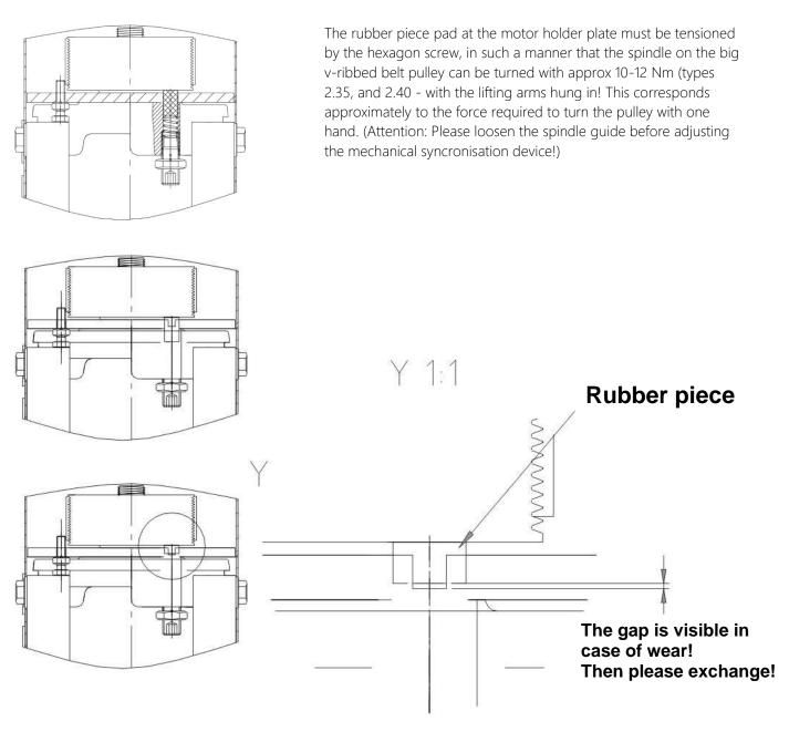
When the motor cover is removed and the lift is without load then the big belt pulley should be rotatable by hand (rough-running). The correct tension of the belt is 194 – 224 Hz.
