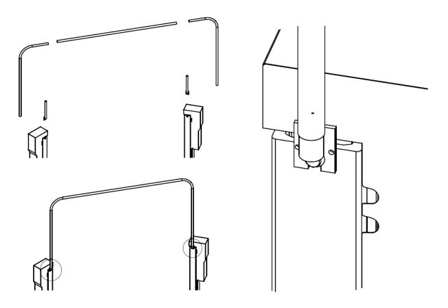
If a control panel is planned at the auxiliary post, the cables for the main switch, the supply, the potentiometers and sockets must be pushed through the pipe of the wire link altogether, starting from the auxiliary post. Then the two halves of the motor cover have to be mounted. Finally, the halves of the motor cover are fixed with pipe clips at the pipe of the wire link.
