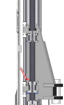
Fig 3 Load nut destroyed
